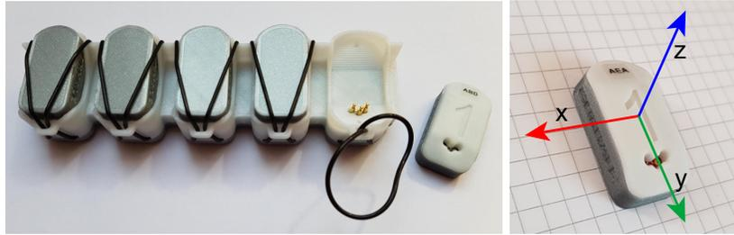
**Figure 1.** Photos of the *PostureSensei™* sensor system. Four of five sensors are sitting in the charger. A single sensor has the dimensions 33 mm × 16 mm × 10 mm and is attached to a person’s back with double sided tape. The right images shows a sensor’s local coordinate system.
